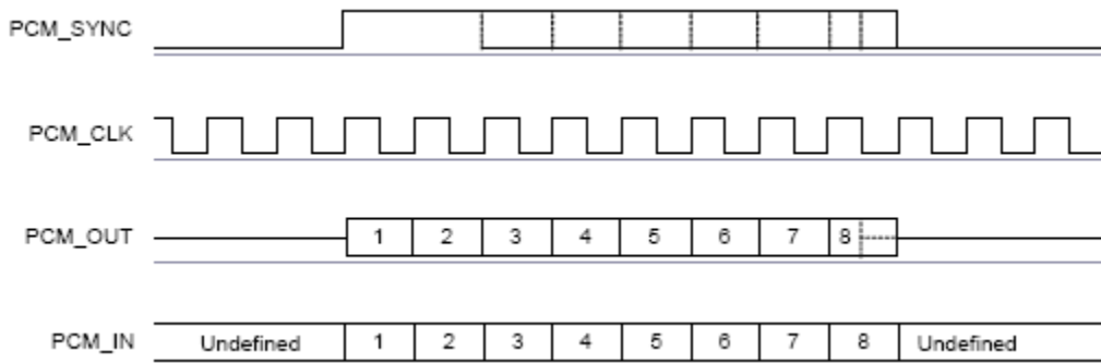
Figure 8: Long Frame Sync (Shown with 8-bit Companded Sample)
